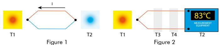
The relationship between the electromotive force and (T1-T2) is not exactly linear. The relationship between the electromotive force and the temperature in degrees is therefore expressed by polynomials  $FEM=f(t^{\circ}C)$ , where the reference junctions of the thermocouples are set to 0°C.
